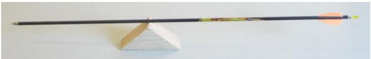
Here the field point is changed out for a 100 grain NAP HellRazor and the balance point is marked with a thin piece of green painter's tape:
